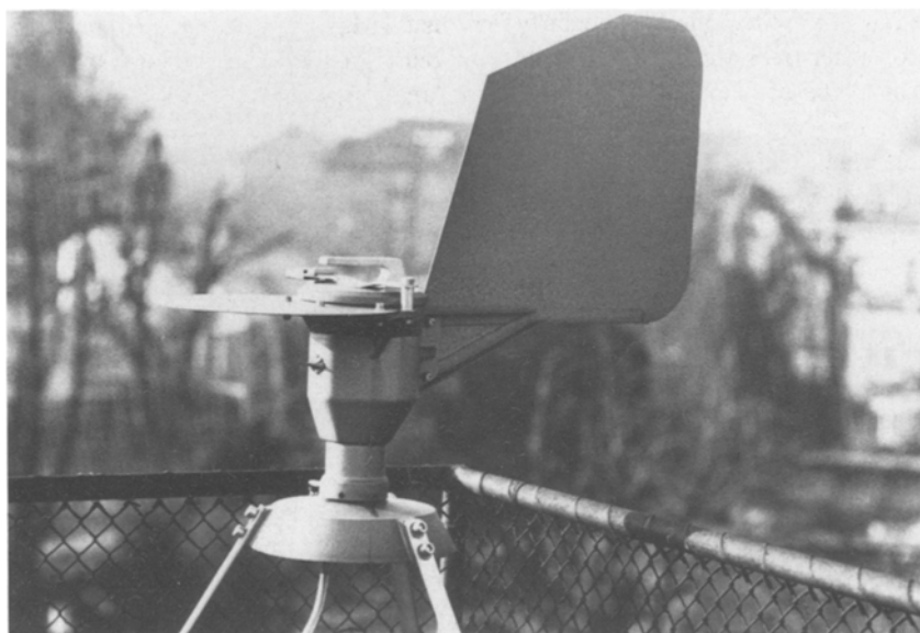
Figure 20. Burkard pollen-and-spore trap (designed by Hirst). From Leuschner 27 . (Photo by R. M. Leuschner.)
